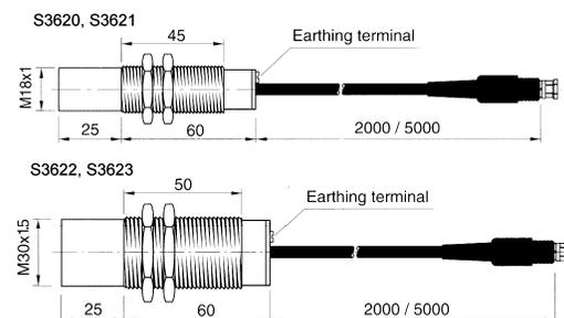
**INSTALLATION INSTRUCTIONS:** If the material to be controlled is in a metallic container, the container and terminal 1 of the amplifier must be grounded. If the container is non-metallic, connect terminal 1 of the amplifier and the earthing terminal on sensor body to ground. The connection wire between the sensor and the amplifier must be separated from the power supply.
